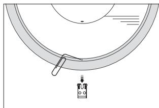
A paper clip can be used to remove the speaker cover.
